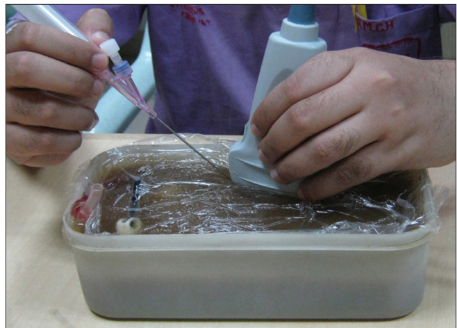
Figure 1: Practice session with gelatin phantom showing position of probe and needle
