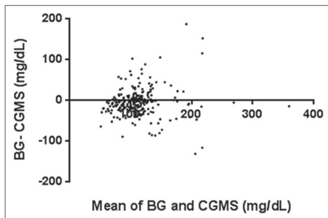
**Figure 3:** Bland–Altman plot of continuous glucose monitoring system (CGMS) versus blood glucose (BG). Mean difference  $- 5.08 \pm 36.6$  mg/dL (limits of agreement  $- 76.6-66.6$ )
