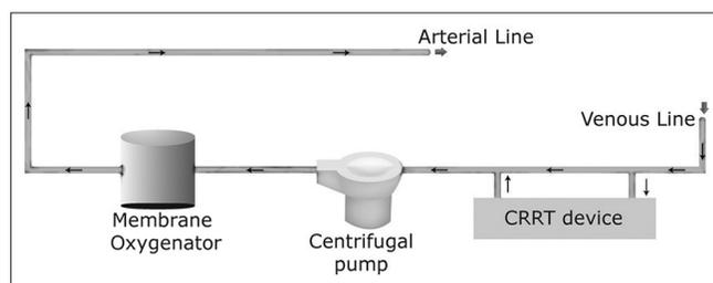
**Figure 1:** Configuration of the system
