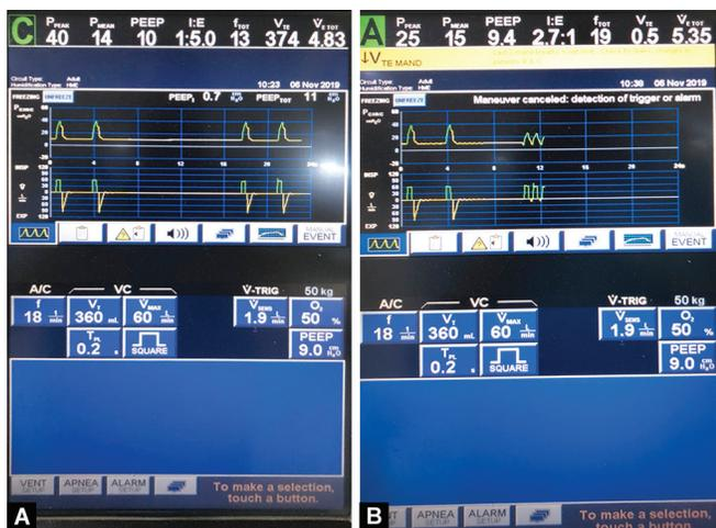
**Figs 1A and B:** (A) End expiratory pause using test lung; (B) Termination of end expiratory pause after opening of suction valve
