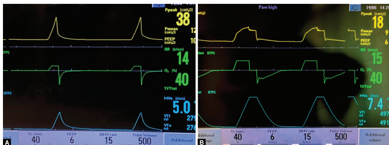
Figs 3A and B: (A) Abrupt rise in inspiratory peak pressure up to 38 cmH 2 O and risk in PEEP of 10 cmH 2 O when the 3L reservoir bag was filled with 800 mL of water. Note the set PEEP was 6 cmH 2 O; (B) Ventilator waveform returns to baseline values after the water-filled reservoir bag was removed from the scavenging system
