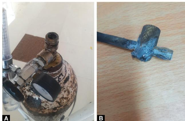
**Figs 1A and B:** (A) The burnt oxygen nozzle; (B) The melted oxygen key
